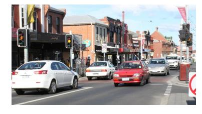
The vehicle amber light can be set to flash after the pedestrian green 'walk' signal has finished, letting drivers go through the crossing as soon as it is clear of pedestrians. This is used to improve traffic flow at narrow crossings, such as a slip lane, or through a single-carriageway shopping zone.
