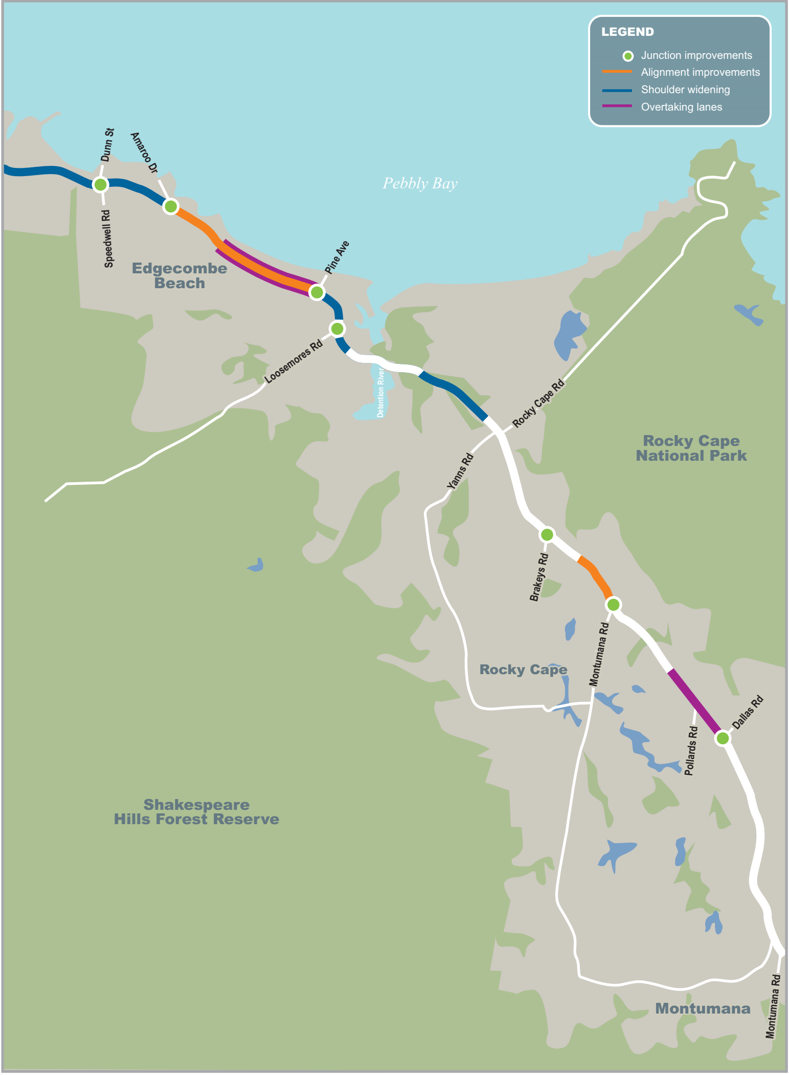
Figure 7.2 CORRIDOR IMPLEMENTATION PLAN - MONTUMANA ROAD TO SPEEDWELL ROAD (Bass Highway, Wynyard to Marrawah)
