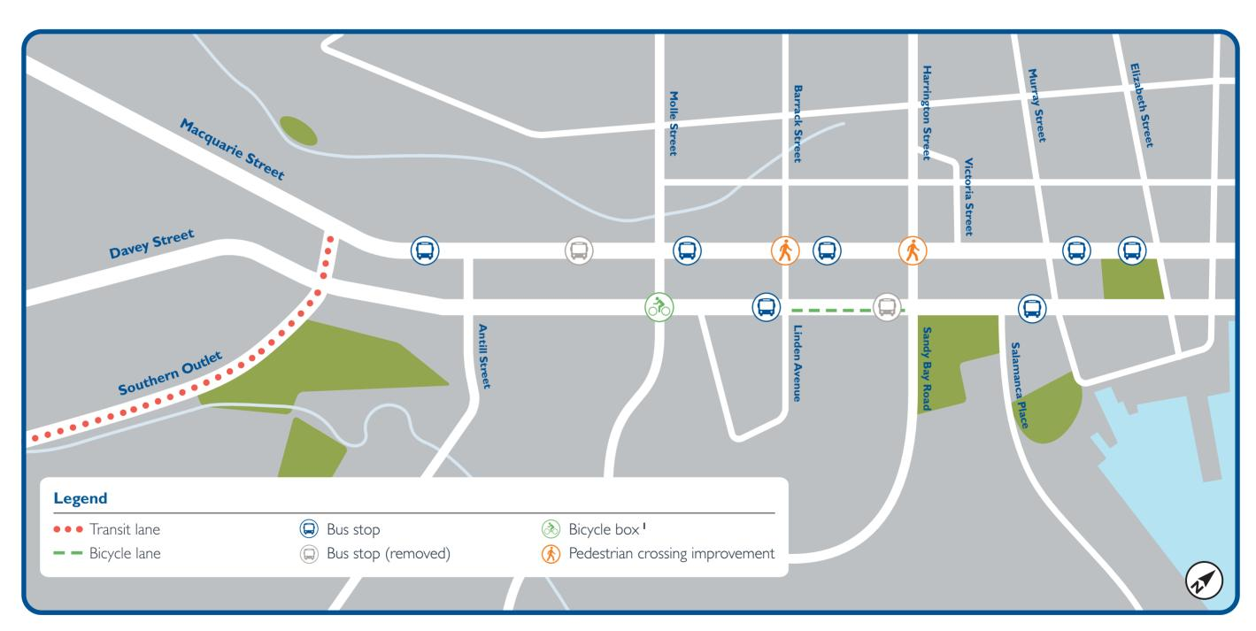
A bicycle box is a a designated area at the head of a traffic lane at a signalised intersection that allows cyclists to move ahead of traffic, improving safety and visibility.
